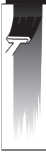
Feathering Technique, use only if stopping in the middle of a log is unavoidable.
